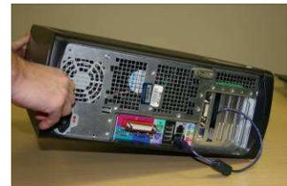
3. **Press and hold the buttons** on the top and the bottom of the PC with both hands, and while doing so **raise the side** of the case.
