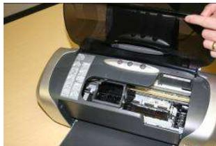
11. With an empty carriage, it pauses four times by the plastic arrow on the body, pointing to each empty position since all four are empty. Each time it pauses, **press the ink button** until the carriage moves to the open position on the right.
