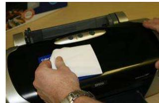
6. **Find the new sticker** packaged with the USB cable, **remove its protective backing**, and carefully **put it into place** where the other sticker was removed.
