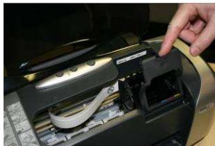
13. **Match the color** on the well with the color of each ink cartridge. **Shake** each cartridge, **open** each in turn, and **press each** into its proper position until it clicks.
