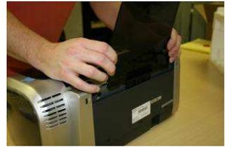
8. **Attach the power cable**, one end into the printer, the other in a power supply, and **press the power button** on the top of the printer. Do not yet plug in the USB cable.
